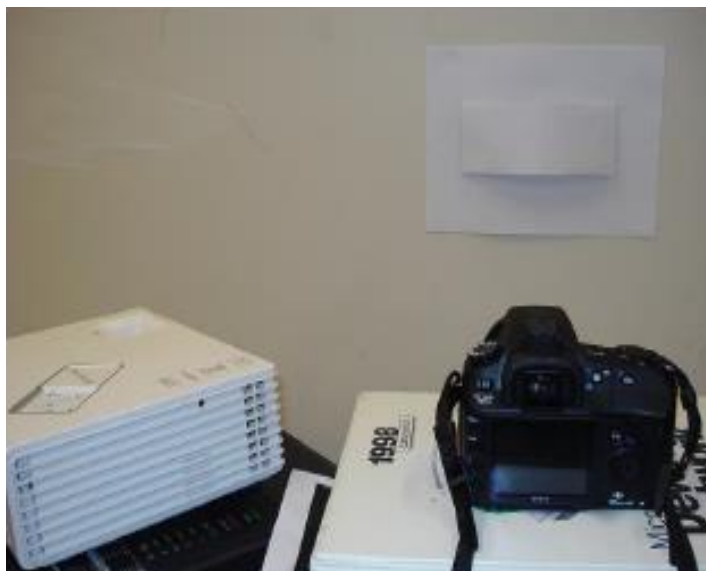
Figure 2.8: Experiment setup of saw tooth projection (Al-Hiary, 2015).
