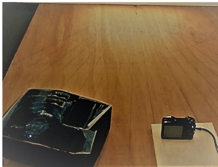
Figure 5.8: The drawn lines on the base board for angles between camera and projector.
