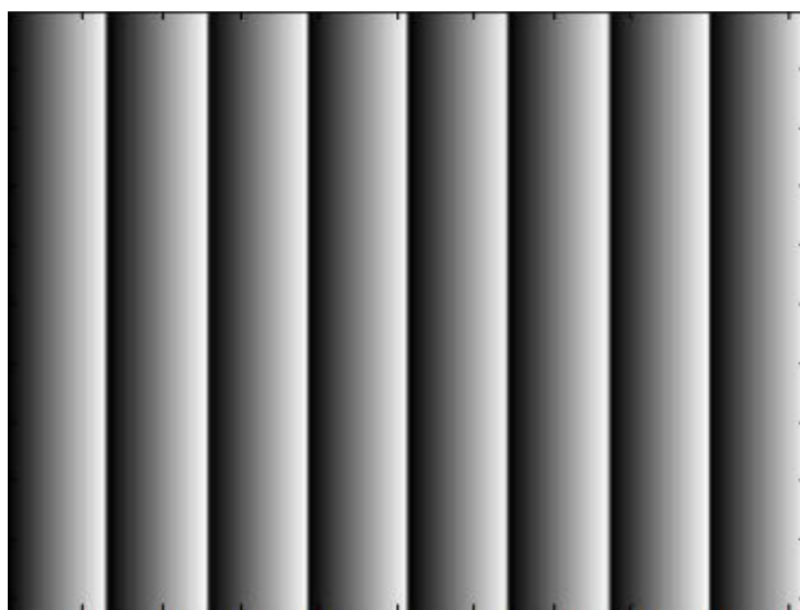
Figure 2.9: Saw tooth fringe patterns (Al-Hiary, 2015).
